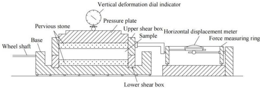
**Figure 3. Strain Controlled Direct Shear Instrument**
