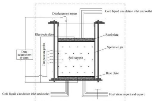
**Figure 2. Schematic Diagram of Freeze-thaw Cycle Test Device**
