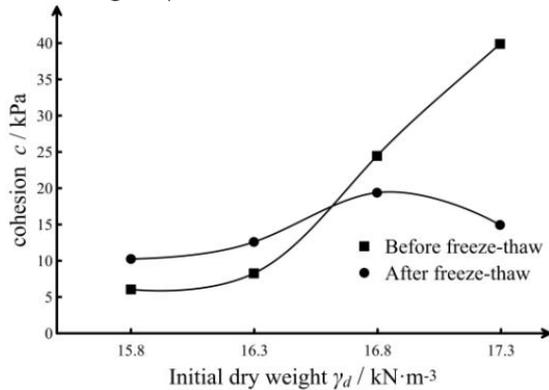
Figure 7. Influence of Different Dry Weight on Cohesion  $c$
