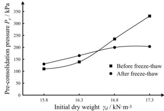
Figure 9. Influence of Different Dry Weight on Pre-consolidation Pressure  $P_c$
