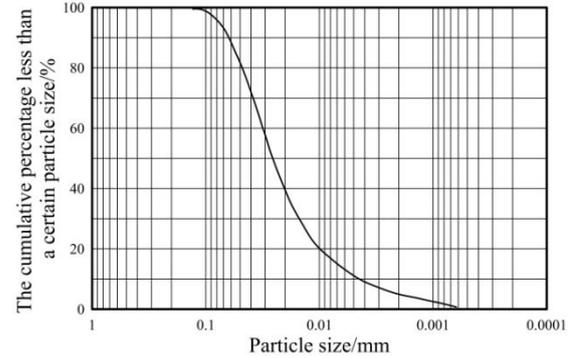
**Figure 1. Grain size Distribution for the Lanzhou Loess**
