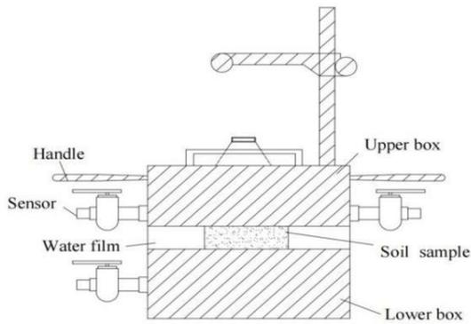
**Figure 4. Coefficient of Resting Lateral Pressure Consolidator Oedometer**
