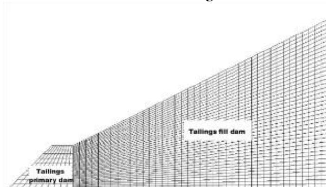
**Figure 1. Numerical Analysis Model of Tailings Dam**
