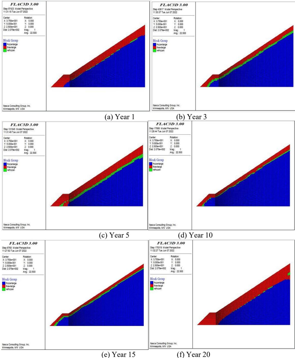
**Figure 2. Thawing Depth Diagram of Different Years Under Operating Condition 1**
