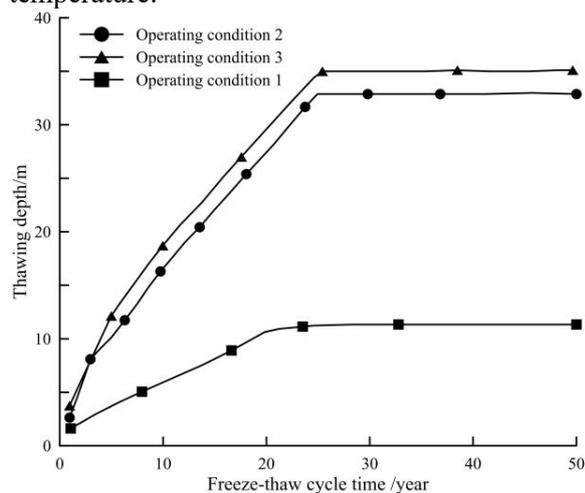
**Figure 3. Comparison of Thawing Depth Under Different Operating Condition.**
