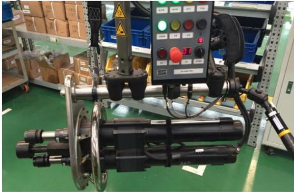
**Figure 4. Status of the Tightening Machine Before Modification**
