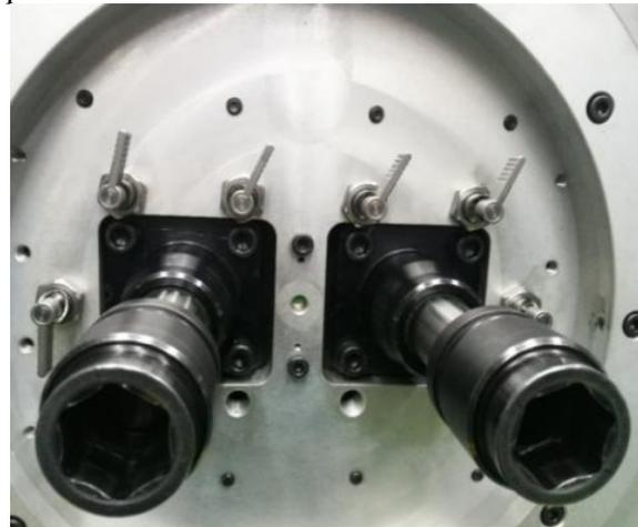
Figure 9. Tightening the Shaft Spacing of 138mm Figure
