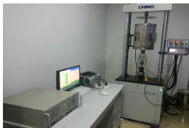
Figure 4. Creep Test Equipment
