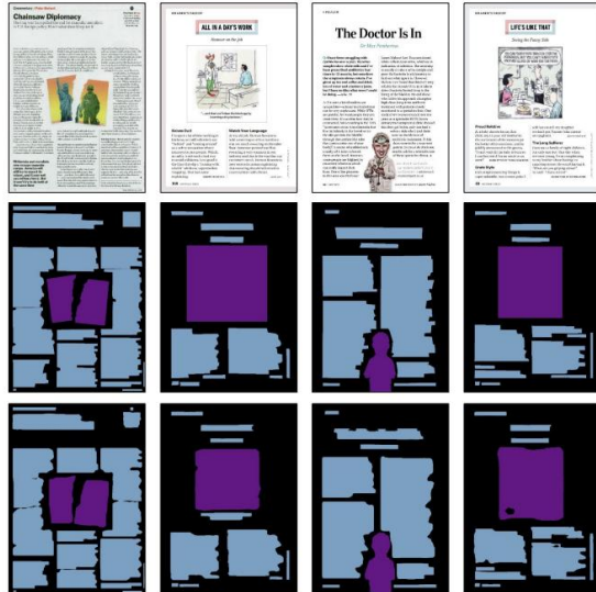
Figure 4. Example Real Documents and Their Corresponding Segmentation on FPD. Top: Original. Middle: Ground-Truth. Bottom: Predictions. Segmentation Label Colors are: Text, Figure, Background
