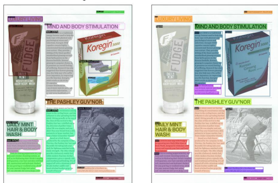
Figure 1. Left: Layout Detected Using Mask R-CNN; Right: the Ground-True of the Layouts. Mask R-CNN Needs to be Trained on the Target Dataset.
