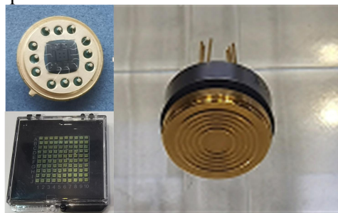
Figure 3. Silicon Piezoresistive Pressure Sensors and Sensitive Structure
