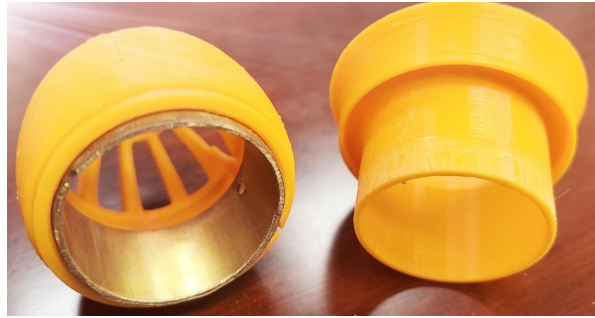
a. Structure of Electrostatic Nozzle b. Photos of Electrostatic Nozzle
