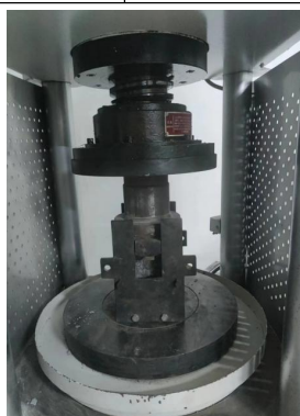
Figure 1. Compressive Strength Test of Standard Self-Healing Concrete Specimen
