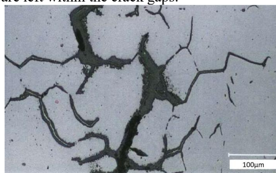
Figure 5. Cracks Filled with Oxides and Unoxidized Filamentous Metals
