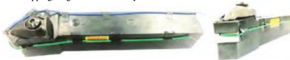
Figure 2. Intelligent Ceramic Cutting Tool for Temperature Monitoring process.
