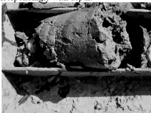
Figure 2. Soil Near The Slip Surface Slip Zone
