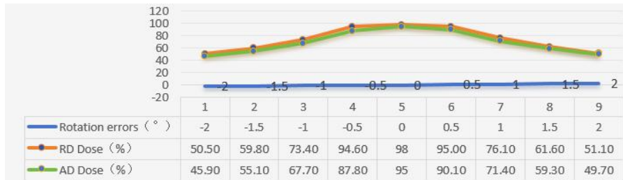
Figure 2. Gamma Pass Rate Curve for Rotational Direction Errors Based on the 3%/3mm Standard
