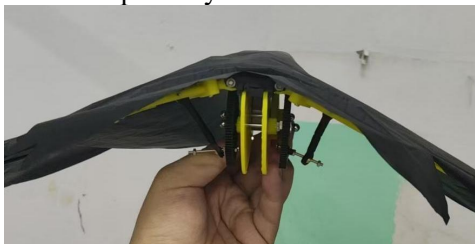
Figure 2. 3D Printing Results of the Bioinspired Robot
