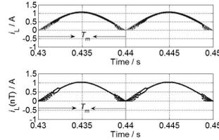
(c) The time domain waveform of the inductor current
