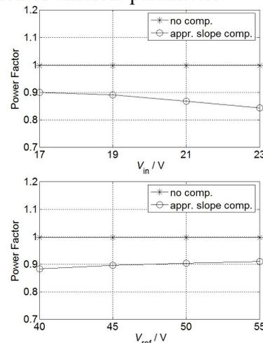
(a) The variation of the input voltage  $V_{in}$  (b) The variation of the reference voltage  $V_{ref}$
