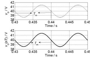
(b) The time domain waveform of the out-put voltage (up)
