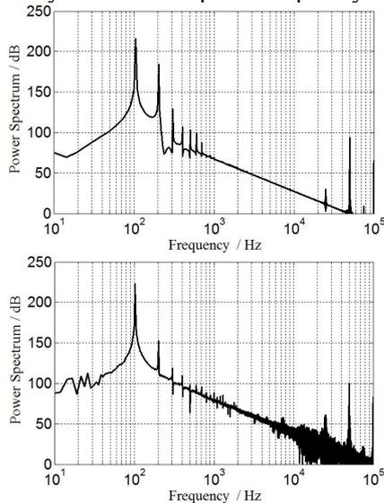
(a) Before the chaos control (correspondent to Figure 1) (b) After the chaos control (correspondent to Figure 2)
