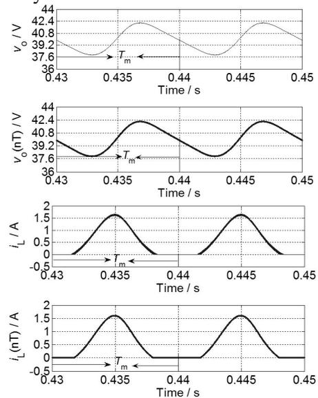
(a) The time domain waveform of the out-put voltage (up); (b) The time domain waveform of the inductor current
