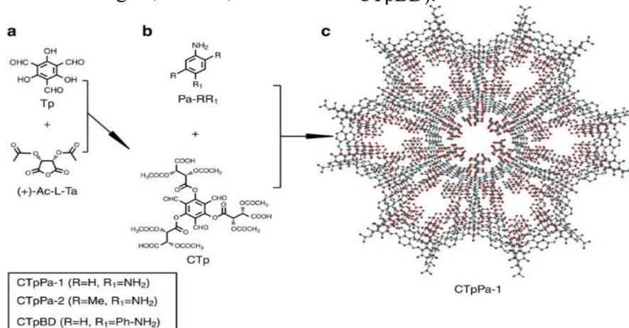
**Figure 4. (a) Synthesis of CTp through the Esterification of Tp and (+)-Ac-L-Ta. (b) Synthesis of Chiral COFs through the Condensation of CTp and Pa-RR1. (c) Graphic view of CTpPa-1 (C, Grey; N, Blue; O, red; H is Omitted for Clarity). [29]**
