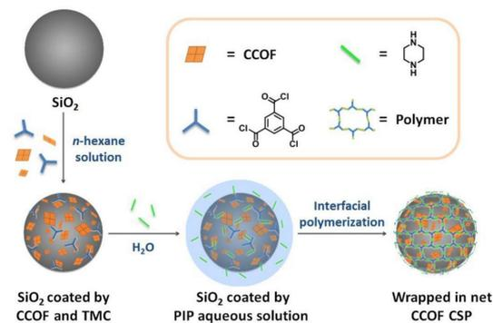
**Figure 2. Fabrication Procedures of the “Wrapped in Net” CCOF CSPs. [27]**
