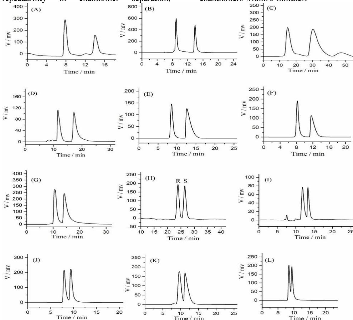
**Figure 6.** HPLC chromatograms obtained using  $\beta$ -CD-COF@SiO<sub>2</sub>-packed column (column A, 25 cm length  $\times$  2.1 mm i.d.) for the separation of racemic compounds: (A) omeprazole, (B) zopiclone, (C) praziquantel, (D) atenolol, (E) flavanone, (F) clenbuterol hydrochloride, (G) trans-stilbene oxide, (H) benzoin, (I) 1-(4-chlorophenyl)ethanol, (J) clenbuterol hydrochloride, (K) 1,1'-bi-2-naphthol, and (L) 2-amino-1-butanol[30].
