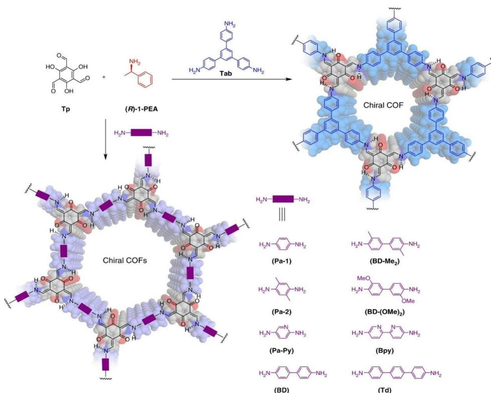
**Figure 3. Schematic Representation of the Synthesis of CCOFs. These CCOFs are Formed from Achiral Precursors by Chiral Catalytic Induction. [28]**
