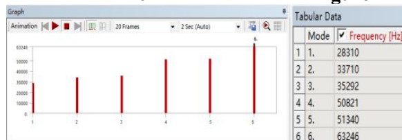
Figure 7. Constrained Modal Frequency of Rolling Bearing(Outer Ring Fixed)
