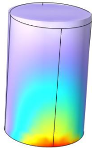
Figure 10. Cloud Diagram of Shear Stress on a Cylinder
