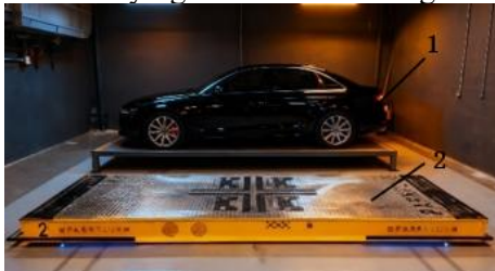
Figure 2. Automatic Parking Robot and Target Vehicle to Be Parked
