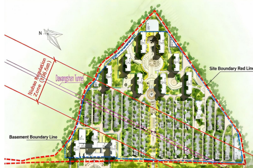
Figure 1. Planar Schematic Diagram of the Relative Position between Plot 1 and the Water Conveyance Line Tunnel
