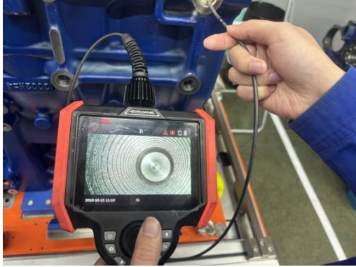
Figure 4. Inspection of the Bolt Holes
