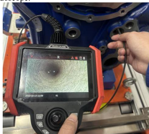
Figure 2. Inspection of the Oil Passage in the Machine Body
