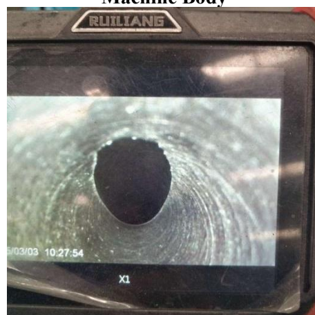
Figure 3. Photo of Burrs in the Oil Passage During the machining process of the engine body, iron filings tend to remain inside the bolt holes, which are difficult to detect with the naked eye. Therefore, an endoscope can be used for inspection. Figure 4 shows the inspection process of the engine body bolt holes. The probe
