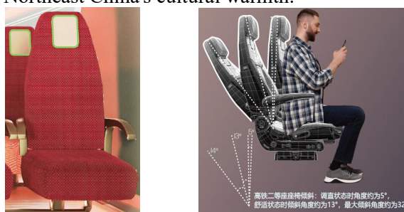
Figure 12. Headrest of the Second-Class Seat in Red and Green Color Scheme (a) and the Angle Adjustment of the Backrest for the Second-Class Seat (b).
