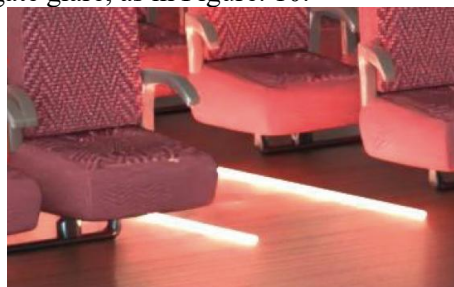
Figure 10. Level Embedded Warning Strip and Guidance Light Under the Seat
