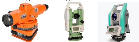
Figure 3. Traditional Monitoring Instruments (from Left to Right: Level, Theodolite, Total Station)
