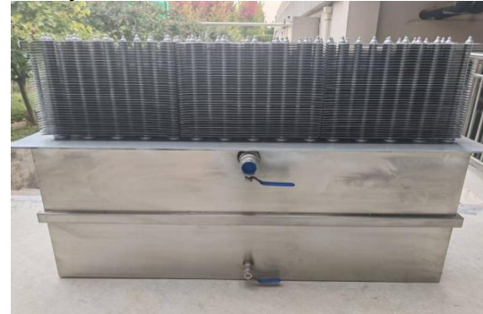
Figure 4. Inverted View of the Waste Heat Recovery Unit
