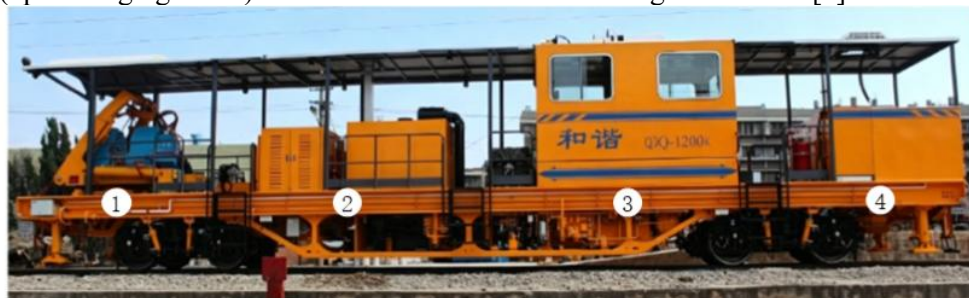
Figure 2. YHGQ-1200K Rail Welding Vehicle: (1) Welding Operation System; (2) Cooling System Compartment; (3) Cab; (4) Power and Auxiliary System Compartment
