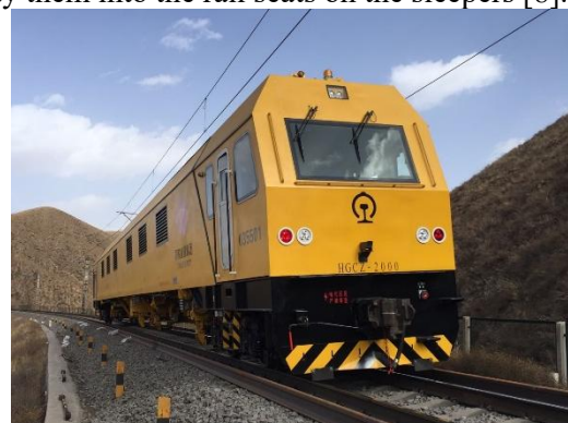
Figure 3. HGCZ-2000 Rail Changing Vehicle
