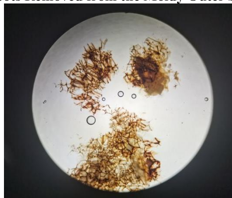
Figure 6. Magnification of Obvious Mildew Spots Removed from the Moldy Outer Side by 100 Times
