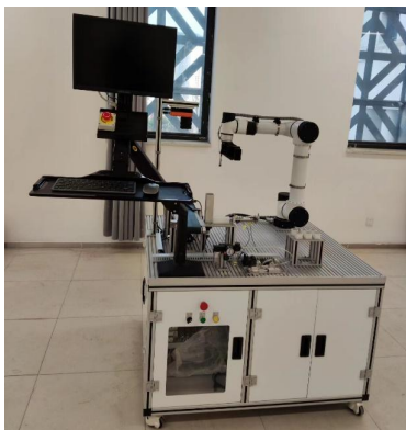
Figure 17. Experimental Platform for Sorting Robot Based on Machine Vision
