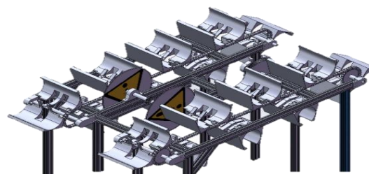
Figure 5. High Speed Root Removal Mechanism
