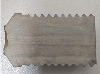
Figure 9. Longitudinal Macrostructure of the Lockbolt
