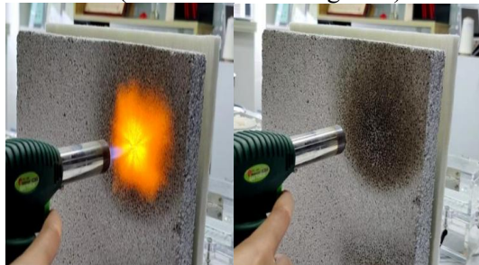
Figure 2. Schematic Diagram of the Flame Resistance Test of SiO 2 Composite Aerogel
